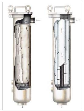
Pictured is a Model 6330. It can hold three 30-in. long cartridges (shown inserted) or a filter bag and support basket (at left). The two 3/4-in. ports at the bottom of the housing are 1) a dirty liquid drain (upper port), and 2) a clean liquid drain (lower port). The dirty liquid drain need not be used when filter bags are employed; if bags are properly removed, no dirt washes off downstream. (The use of a liquid displacer makes this easier to do.)
